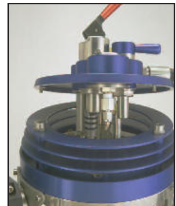
▲ Sirocco Manifold Block
