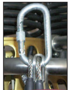
▲ Rigging Of Frame Type 'C'
